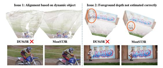
Figure 2: **Limitation of DUSt3R on dynamic scenes.** Left: DUSt3R aligns the moving foreground subject and misaligns the background points as it is only trained on static scenes. Right: DUSt3R fails to estimate the depth of a foreground subject, placing it in the background.
