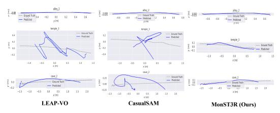
Figure A3: **Camera pose estimation comparison on the Sintel dataset.** The trajectories are plotted along the two axes with the highest variance to capture the most significant motion. The predicted trajectory (solid blue line) is aligned to match the ground truth trajectory (dashed gray line). Our MonST3R is more robust at challenging scenes, "temple\_3" and "cave\_2" (the last two rows).
